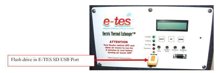
4. Press and hold both the UP button and DOWN button while your turn the power switch ON.
