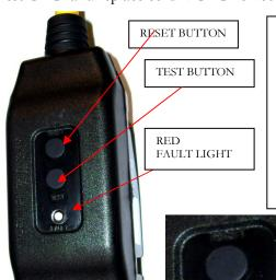
When the GFCI cord is connected to the 120vac outlet, push the RESET Button. Then, push the TEST button to test the GFCI.
