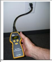
USE CIRCUIT ANALYZER TO CHECK CIRCUIT LOAD
