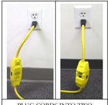
PLUG CORDS INTO TWO OUTLETS ON TWO SEPARATE CIRCUITS
